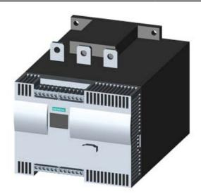
SIRIUS SOFT STARTER, VALUES WITH 460 V, 50 DEG., STANDARD: 180A, 125HP, INSIDE-DELTA CIRCUIT 3: 312A, 250HP, 200-460 V AC, 115 V AC, SCREW TERMINALS
